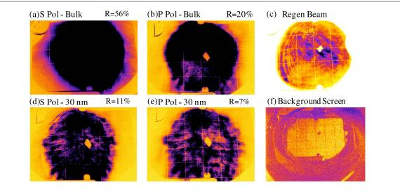
**Figure 4.** Reflected beam profiles of the fundamental laser pulse for a variety of conditions. (a), (b), (d), (e) The same images as figure 2, with the same color scale. The color scale is taken such that any light above three standard deviations of the background noise appears black. (c) The reflectivity profile from the low-power amplified beam. (f) The background shot with no laser interaction.
