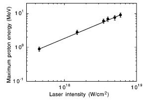
FIG. 1. Maximum proton energy in the forward direction as a function of laser intensity for 6  $\mu$ m Mylar foil.
