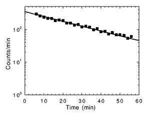
FIG. 3. Measured decay of radioactivity vs the time for the  $^{10}\text{B}(d,n)^{11}\text{C}$  reaction (squares). The solid line corresponds to the theoretical result and demonstrates  $\sim 20$  min half-life of  $^{11}\text{C}$ .
