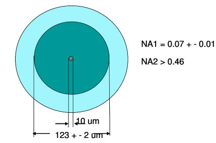
The DCF used in this study has a numerical aperture of 0.46, which is smaller than that of a double clad photonic crystal fiber we have used previously DCPCF, (Ye, et al, *Proceedings of the SPIE*, 2005. 5700: p. 23-27). Although the collection efficiency is not quite as high as for the DCPCF, it still provides significant improvement over traditional single-clad fibers.
