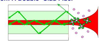
Enhancing Fiber-Optic Sensing Technique Using a Dual-Core Fiber J. Y. Ye, T. B. Norris, M. T. Myaing, T. Thomas, J. R. Baker, Jr. Patent filed in December, 2002.
