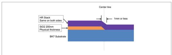
**Figure 1.** Schematic of the mirror used to induce pi phase shift. Beam incident on the portion of the mirror without the additional  $SiO_2$  layer travels 400 nm ( $\lambda/2$ ) farther.
