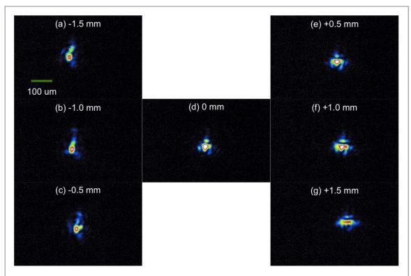
Figure 2. Representative images of the energy distribution within a single focal spot throughout the confocal length of the f/20 focusing optic. 0 mm denotes the position of best focus. Positive numbers denote positions after focus and vice versa for negative numbers.
