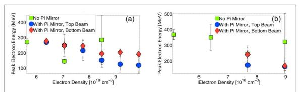
Figure 9. Maximum electron energy versus density for beams generated using the (a)  $2.5\%~N_2$  gas mixture and (b) pure He gases, averaged over multiple shots. The designation of 'top' and 'bottom' correspond to the orientation of the beams on the detector.
