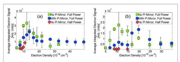
**Figure 7.** Integrated electron signal versus density for beams generated using the (a) 2.5% N<sub>2</sub> gas mixture (b) pure He gas. The  $\pi$  phase shift mirror was used to generate dual electron beams. This effect is more pronounced for the pure He gas.
