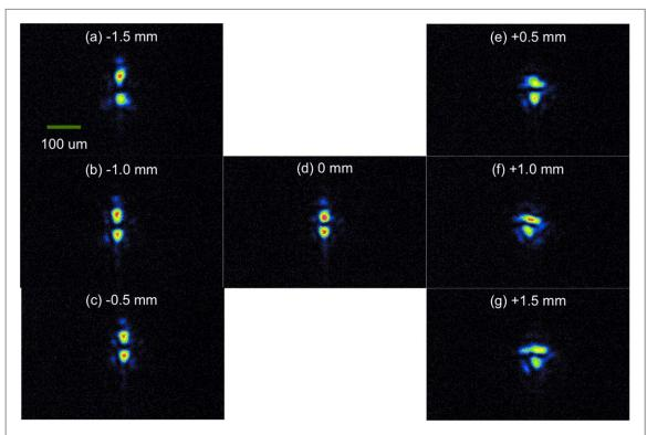
**Figure 3.** Representative images of the energy distribution within dual focal spots, generated using a coated mirror, throughout the confocal length of the f/20 focusing optic. A slight asymmetry in the energy distribution (weighted towards the top beam) can be seen for the dual focal spots. 0 mm denotes the position of best focus. Positive numbers denote positions after focus and vice versa for negative numbers.
