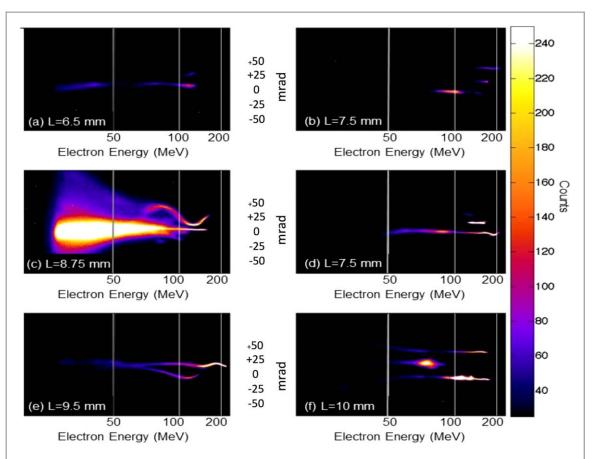
Figure 6. (a)—(c) Energy spectra of dual electron beams. Interaction between the electron beams led to trajectory crossing between the beams and increased transverse oscillations. (d)—(f) Injection and acceleration of a third electron beam occurs due to the coherent superposition between the diffracted parts of the original two focal spots as demonstrated in the simulations. Gas cell length is indicated in each figure (note that 200 pixels corresponds to  $\sim$ 3°).
