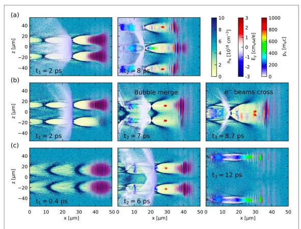
Figure 10. Snapshots of simulation results at different time steps. (a) 3D simulations of two 50 TW, 30 fs laser pulses separated by 30  $\mu$ m in plasma having an electron density of 6  $\times$  10<sup>18</sup> cm<sup>-3</sup>. (a) Identical 3D simulations as in (b) with perpendicularly polarized beams (c) identical 3D simulations as in (a) with  $\pi$  phase shift between the two beams. The subpanels of (a)–(c) show the simulations at different times.
