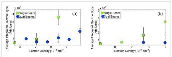
Figure 8. Integrated electron signal comparison between single (full energy) and dual electron beams for the (a)  $2.5\% N_2$  gas mixture and (b) pure He gas. The data is shown in finer detail than in figure 7 and it is clear than the dual beams do not in general produce more charge than the single beam at full power.
