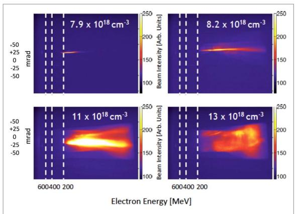
**Figure 5.** Typical energy spectra of electron beams generated using a single focal spot for differing plasma densities. The beams in both columns were created with 55 TW of laser power and a 3 mm gas cell.
