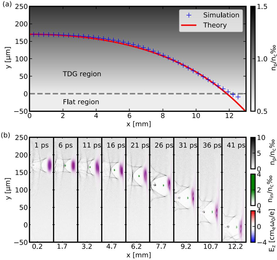
FIG. 1. (a) Plasma density distribution and the laser pulse trajectory predicted by the theoretical model (red line) and from the simulation (blue crosses). (b) Snapshots of the evolution of the laser pulse, the background plasma density, and the injected electron beams.
