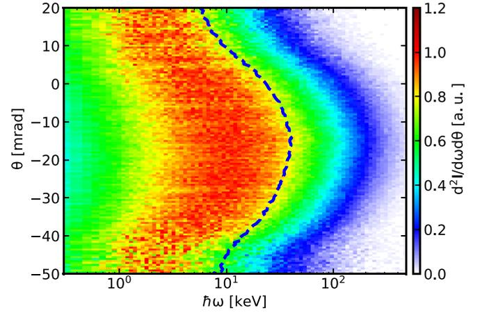
FIG. 2. Streaked angular spectrum at the end of the simulation. For each angle, the spectrum was normalized to its maximum. The blue dashed line represents the critical photon energy for each angle, fitted with the synchrotron spectrum.
