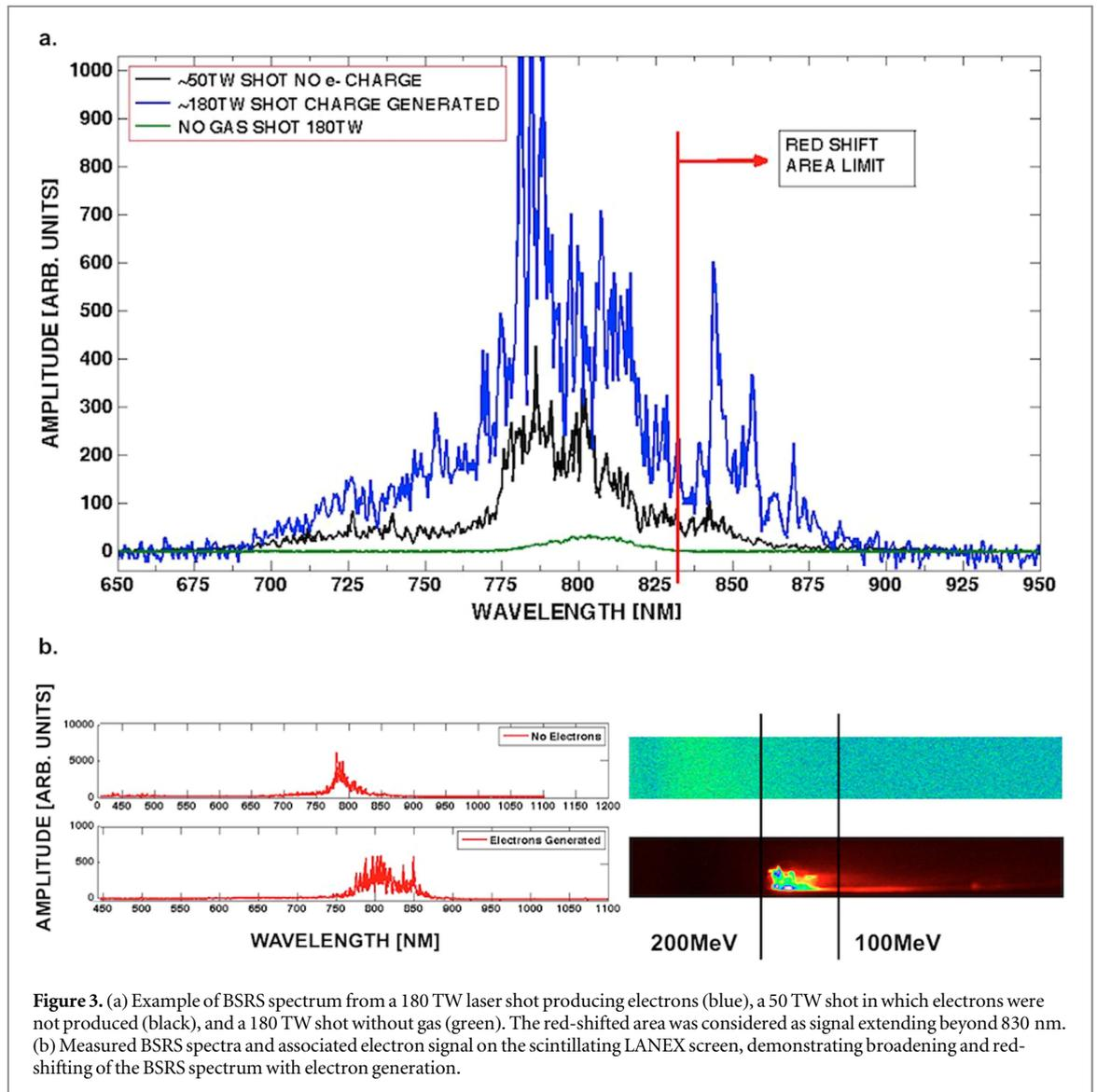
**Figure 3.** (a) Example of BRS spectrum from a 180 TW laser shot producing electrons (blue), a 50 TW shot in which electrons were not produced (black), and a 180 TW shot without gas (green). The red-shifted area was considered as signal extending beyond 830 nm. (b) Measured BRS spectra and associated electron signal on the scintillating LANEX screen, demonstrating broadening and red-shifting of the BRS spectrum with electron generation.
