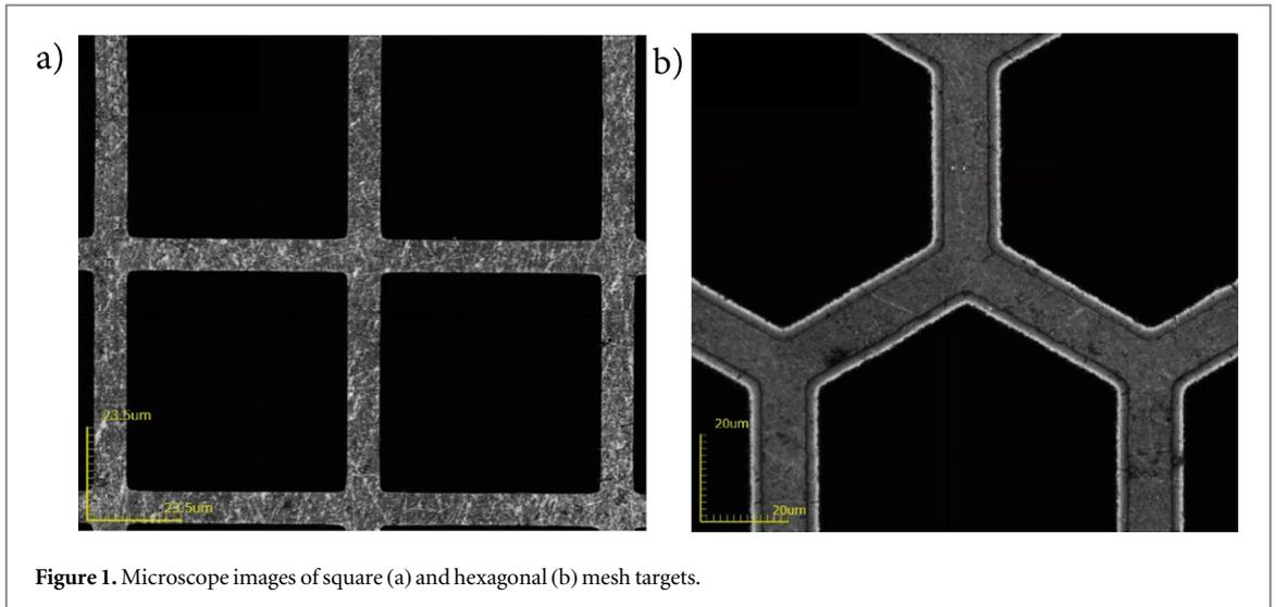
Figure 1. Microscope images of square (a) and hexagonal (b) mesh targets.
