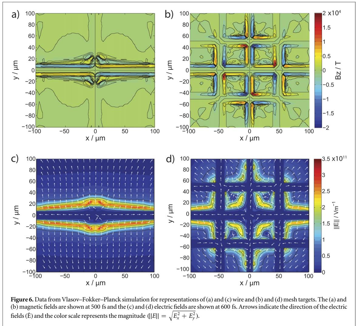
**Figure 6.** Data from Vlasov–Fokker–Planck simulation for representations of (a) and (c) wire and (b) and (d) mesh targets. The (a) and (b) magnetic fields are shown at 500 fs and the (c) and (d) electric fields are shown at 600 fs. Arrows indicate the direction of the electric fields ( $\vec{E}$ ) and the color scale represents the magnitude ( $\|E\| = \sqrt{E_x^2 + E_y^2}$ ).
