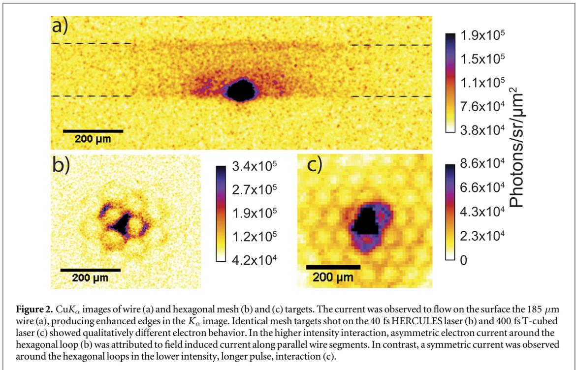
in figure 2(a) demonstrated that the current was flowing on the surface of the  $185 \mu\text{m}$  wire. This provided experimental corroboration of simulations of laser induced electron transport in  $40 \mu\text{m}$  wires which predict that the bulk of the current traveled along the wire surface [27].
